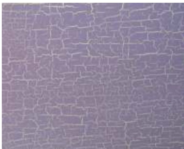
Overpaint by brush with coloured 10% diluted water paint (binder content 20%).
